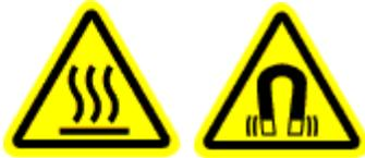
Do not wear clothing that is made with metallic pocket rivets, waist band buttons, pocket buttons, and zippers when operating the Mini-Ductor™ II. The Mini-Ductor™ II can heat such metallic items very quickly and cause serious burns or even ignite clothing.
