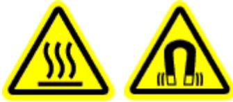
Remove all loose coins, metallic tokens, keys, chains, pocket knives, miniature tools, or any other metallic object in or on your clothing before operating the Mini-Ductor™ II. Do not replace these items until you are finished using the Mini-Ductor™ II. The Mini-Ductor™ II can heat these metallic objects very quickly and cause serious burns or even ignite clothing.
